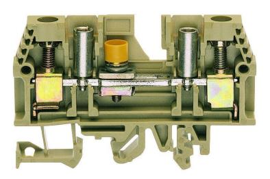
Test disconnect terminal, Screw connection, Mounting type:Mounting rail TS 35/7.5 and TS 32, Rated cross-section: 10 mm², Width: 8 mm, Colour: Beige
