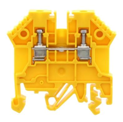
Feed-through terminal, Screw connection, Mounting type:Mounting rail TS 35/7.5 and TS 32, Rated cross-section: 2.5 mm², Width: 5 mm, Colour: Yellow
