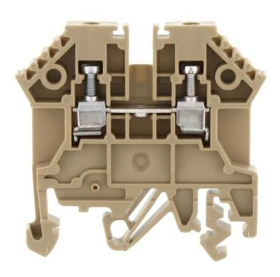
Ex feed-through terminal ATEX-certified, Screw connection, Mounting type:Mounting rail TS 35/7.5 and TS 32, Rated cross-section: 2.5 mm², Width: 5 mm, Colour: Beige
