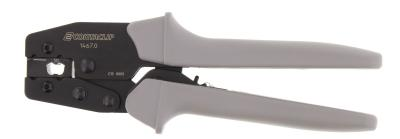
Crimping tool for crimping wire-end ferrules with and without plastic collars. Cross-section range: 50 mm<sup>2</sup>. Easy to use, Auto-lock for proper and complete crimping, Wire can be fed in from the side, Self-opening with built-in spring.
