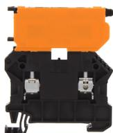
Fuse-disconnect terminal, Screw connection, Mounting type: Mounting rail TS 35/7.5, Rated cross-section: 4 mm<sup>2</sup>, Width: 6.1 mm, Colour: Black
