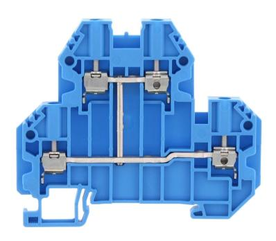
Double-level terminal, Screw connection, Mounting type: Mounting rail TS 35/7.5, Rated cross-section: 2.5 mm², Width: 5.1 mm, Colour: Blue
