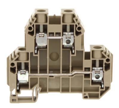
Double-level terminal, Screw connection, Mounting type: Mounting rail TS 35/7.5, Rated cross-section: 10 mm², Width: 10.1 mm, Colour: Beige
