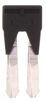
Insulated cross-connector, No. of poles: 2, Mounting type: Plug in, Width: 9.9 mm, Rated cross-section: 2.5 mm<sup>2</sup>, Colour: Black
