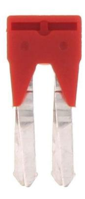
Insulated cross-connector, No. of poles: 2, Mounting type: Plug in, Width: 9.9 mm, Rated cross-section: 2.5 mm², Colour: Red
