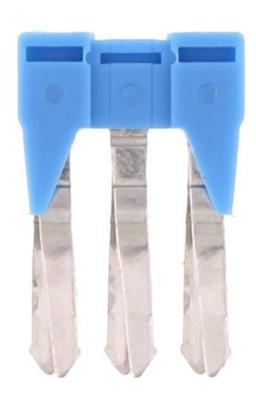
Insulated cross-connector, No. of poles: 3, Mounting type: Plug in, Width: 15 mm, Rated cross-section: 2.5 mm², Colour: Blue
