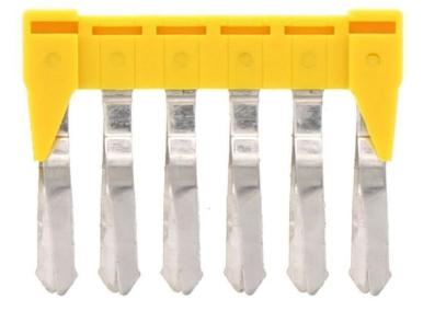
Insulated cross-connector, No. of poles: 6, Mounting type: Plug in, Width: 30.3 mm, Rated cross-section: 2.5 mm<sup>2</sup>, Colour: Yellow
