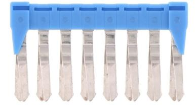
Insulated cross-connector, No. of poles: 8, Mounting type: Plug in, Width: 40.5 mm, Rated cross-section: 2.5 mm<sup>2</sup>, Colour: Blue
