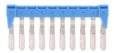
Insulated cross-connector, No. of poles: 10, Mounting type: Plug in, Width: 50.7 mm, Rated cross-section: 2.5 mm², Colour: Blue
