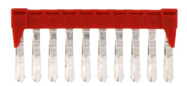
Insulated cross-connector, No. of poles: 10, Mounting type: Plug in, Width: 50.7 mm, Rated cross-section: 2.5 mm², Colour: Red
