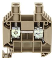
Feed-through terminal, Screw connection, Mounting type: Mounting rail TS 35/7.5, Rated cross-section: 16 mm<sup>2</sup>, Width: 12.1 mm, Colour: Beige
