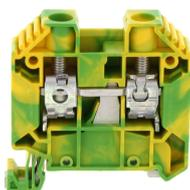
Protective earth terminal, Screw connection, Mounting type: Mounting rail TS 35/7.5, Rated cross-section: 16 mm<sup>2</sup>, Width: 10 mm, Colour: Green-yellow
