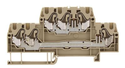
Double-level terminal, Push-in connection, Mounting type: Mounting rail TS 35/7.5, Rated cross-section: 2.5 mm², Width: 5.1 mm, Colour: Orange
