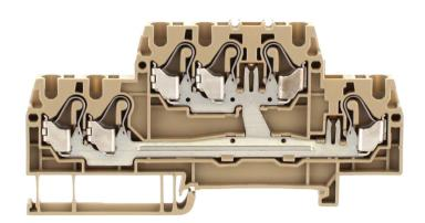
Double-level terminal, Push-in connection, Mounting type: Mounting rail TS 35/7.5, Rated cross-section: 2.5 mm², Width: 5.1 mm, Colour: Blue
