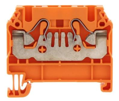
Feed-through terminal, Push-in connection, Mounting type: Mounting rail TS 35/7.5, Rated cross-section: 4 mm<sup>2</sup>, Width: 6.1 mm, Colour: Orange
