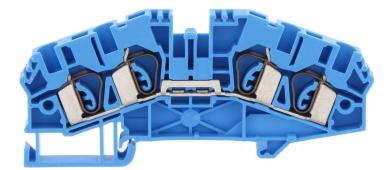
Feed-through terminal, Tension-spring connection, Mounting type: Mounting rail TS 35/7.5, Rated cross-section: 4 mm<sup>2</sup>, Width: 6.1 mm, Colour: Blue
