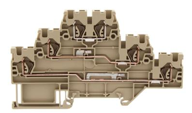
Three-level initiator terminal | Multi-wire terminal, Tension-spring connection, Mounting type: Mounting rail TS 35/7.5, Rated cross-section: 2.5 mm², Width: 5.1 mm, Colour: Beige
