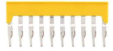
Insulated cross-connector, No. of poles: 10, Mounting type: Plug in, Width: 58.9 mm, Rated cross-section: 4 mm<sup>2</sup>, Colour: Yellow
